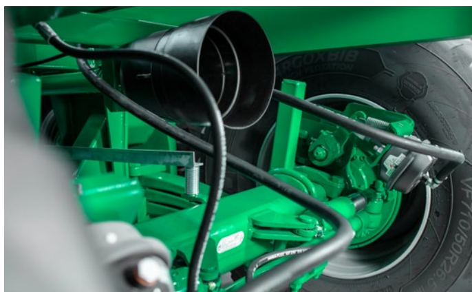
The heavy BPW bogie chassis with ALB controller is part of the standard scope of the HS 220.
