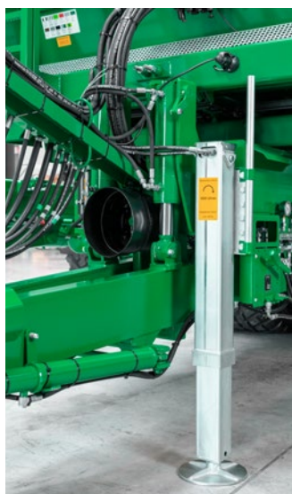
Picture left: The hydraulic support foot allows easy attachment and removal of the spreader.
