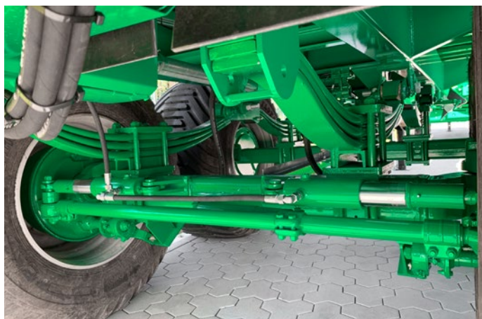
Picture top: The optional self-steering axle in the heavy-duty version.
